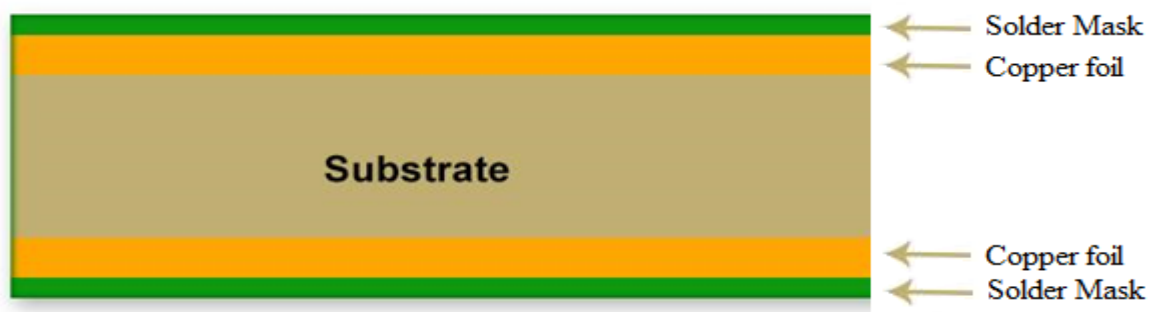
Figure 13.3 Double Layer PCB
