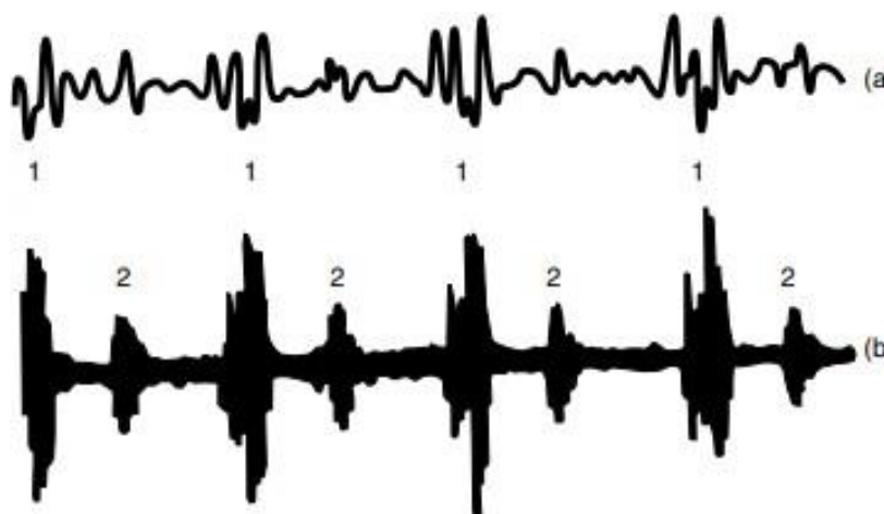
Fig. 9.3 Fetal phonocardiogram: (a) unfiltered heart sound, (b) filtered heart sounds (Copyright--Handbook of biomedical instrumentation by R.S. Khandpur (Third edition))
