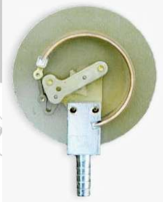
Fig 4.3 Mechanical side with Bourdon tube
